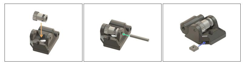
• Place the idler gear into the *extruder\_idler*. Note the orientation of the teeth.
