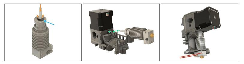
(i) Hotend wires are not visible on these images. Use the heatblock to orientate the hotend correctly.
