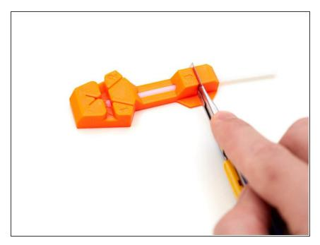
Keep the PTFE inside the jig and trim the length. Make sure the PTFE is fully seated and does not move while making the cut.
