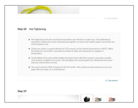
Hot-tighten the Hemera nozzle to 3Nm at 285°C. Follow the official instructions of the E3D Hemera assembly guide here (step 18): <a href="https://e3d-online.dozuki.com/Guide/02+-...">https://e3d-online.dozuki.com/Guide/02+-...</a>
