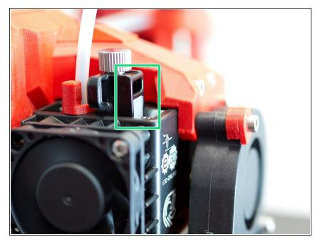
As a starting point to adjust the extruder tension, E3D recommends to rotate the tensions screw until the white part is flushed with the front of the black part.
