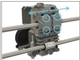
Clamp the extruder on the top and bottom linear bearings of the X axis
