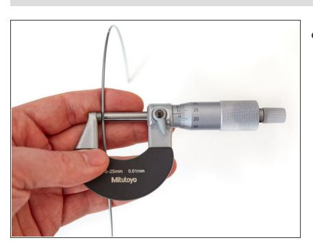
Follow our "Extrusion multiplier" guide here: <u>8. Extrusion multiplier</u> and filament diameter
