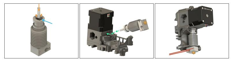
(i) Hotend wires are not visible in these images. Use the heatblock to orientate the hotend correctly.
