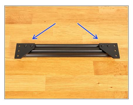
Repeat the previous step on the other side of the 290mm extrusion.
