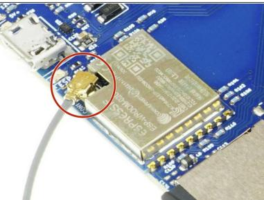
The antenna connector is quite a tight fit, and is not intended for frequent connecting/disconnecting!
