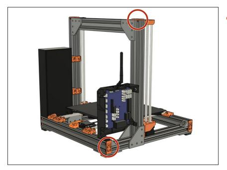
Re-attach the end caps on both the left Z extrusions and the extrusion on the back of the XY-frame.
