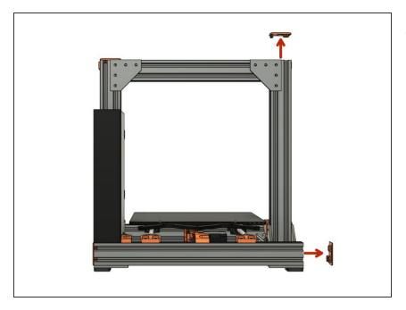
Remove the Z end cap on the left Z extrusion and on the left end of the back XY-frame extrusion (left when standing in front of the printer).
